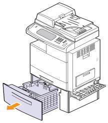
6 Remove the paper in the direction shown. Pull it out gently and slowly in order to avoid tearing the paper.
